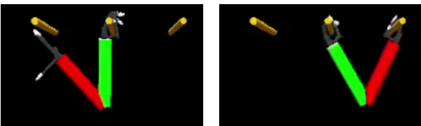
Fig. 1. Initial and final configurations at the start and end of a single brachiation cycle.
